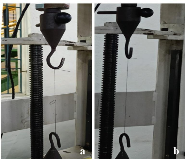
Figure 1. (a) Knot pull test by tensile tester; (b) Straight pull test by tensile tester
