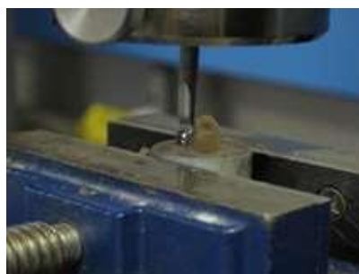
Figure 1. Specimen under shear bond strength testing
