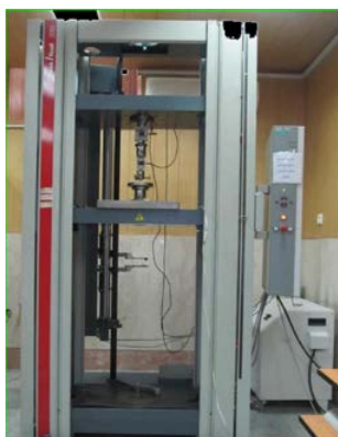
Figure 2. Compressive load application to the central fossa of the core at a 90° angle relative to the longitudinal axis of the tooth at a crosshead speed of 0.5 mm/minute using the Instron machine (Z050, Zwick/Roell, Ulm, Germany)
