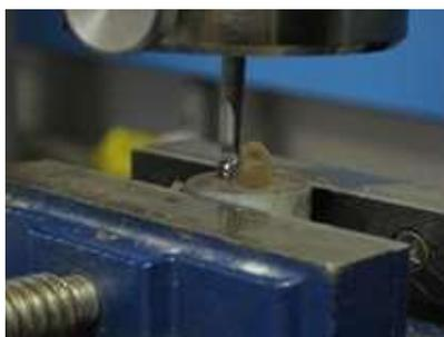
**Figure 1. Specimen under shear bond strength testing**
