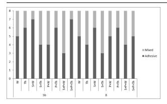
**Figure 4.** Failure modes observed in different experimental groups: (a) mixed failure, (b) adhesive failure. W: storage in water for 24 h, Th: thermocycling, S: silane application, P: argon plasma application, Sb: sandblasting, B: bur roughening
