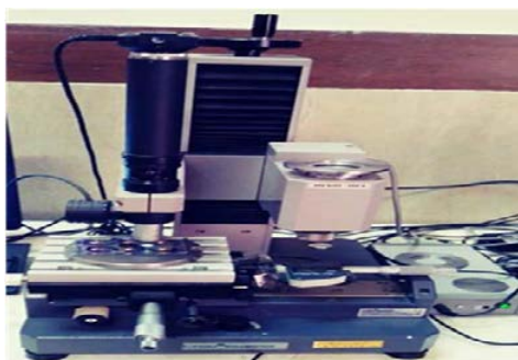
Figure 5. Placement of samples in the Vickers testing machine
