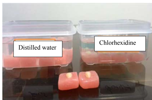
Figure 3. Immersion of samples in the solutions: Chlorhexidine (right) and distilled water (left)
