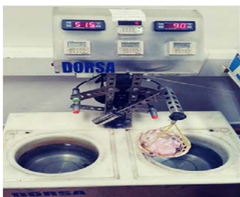
Figure 4. Placement of samples in the thermocycling unit
