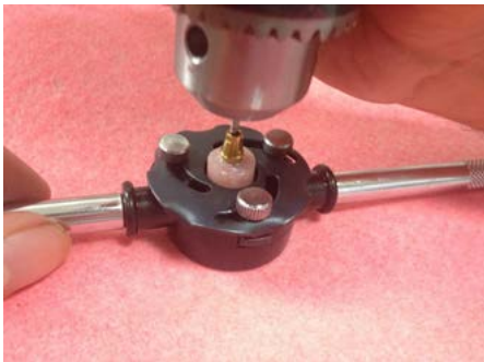
Figure 2. Measuring the removal torque value (RTV) by a torque-meter
