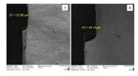
Figure 1:SEM micrographs showing the depth (μm) of erosion. (A): 15% HCl/90 seconds. (B): 18% HCl/90 seconds
