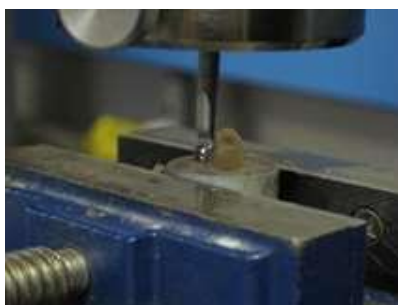
Figure 1. Specimen under shear bond strength testing
