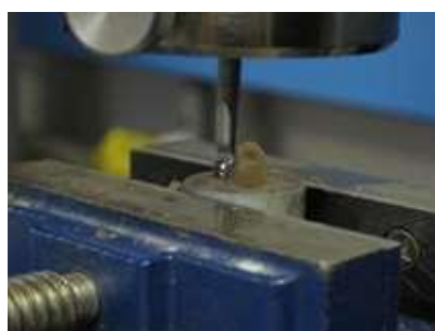
Figure 1. Specimen under shear bond strength testing
