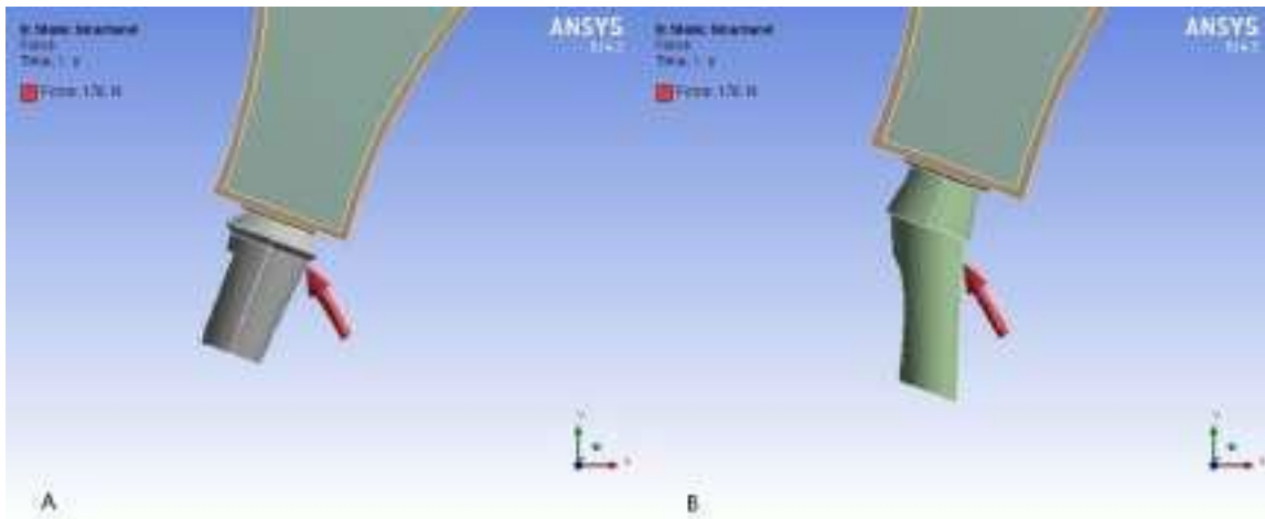
Figure 2- Schematic view of the direction of load application. A: Straight abutment. B: Angled abutment
